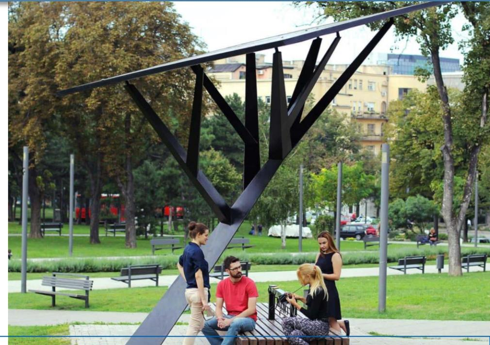
*People charge their phones on a solar-powered smart bench in Belgrade, designed by the Serbian start-up Strawberry Energy. It provides users with free Wi-Fi and battery-charging services, as well as data on air quality, air temperature and noise levels.*
